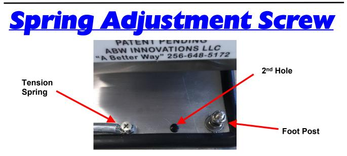
The cone table has tension on the shaper cone by use of the tension spring. Depending upon the type of batter/cone recipe being used, less tension may be needed. You can move the spring to the next screw position, located under the black hole plug–-or to the 3<sup>rd</sup> foot post–where a lock nut has been provided. Adjust as necessary for your situation. NORMALLY NO ADJUSTMENT IS NEEDED HERE! TALK WITH US FIRST! Usually all adjustments for quality cone production are made with the Rail Lock.
