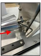
5. Reinstall the matching size shaper plate (for small or large cone). Before tightening Phillips screws, align shaper plate over cone shaper tool–all sides should be equal & centered. Tighten Phillips screws.
