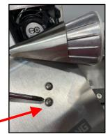
6. Reattach tension spring to spring tension mount. Tighten nut only to cover top of bolt. Now run cones as normal with your new sized cone shaper.
