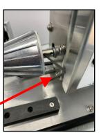
4. Insert the desired cone shaper (small or large) and insert into the coupler firmly. Re-tighten allen screw tightly, use pliers if required.
