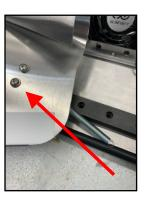
3. Insert supplied Allen Wrench into the left Allen Nut, turning to counter clockwise to loosen. Only a turn or two is needed. Then pull front cone shaper tool, to the left, to remove from the coupler.
