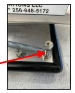
2. Slide cone shaper to the left, down the rail, so the unit is out of the way. Then remove the two Phillips head screws in the shaper plate and set plate aside.
